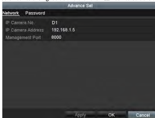
Figure 2. 25 Network Configuration of the Camera
